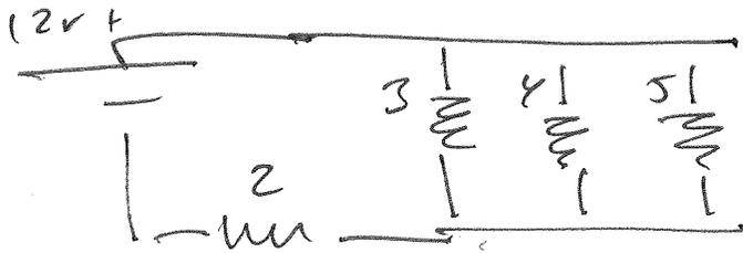
$$(1) \quad \frac{1}{3} + \frac{1}{4} + \frac{1}{5} = \frac{1}{R_{net}} = \frac{20}{60} + \frac{15}{60} + \frac{12}{60} = \frac{47}{60} = \frac{1}{R_{net}}$$
