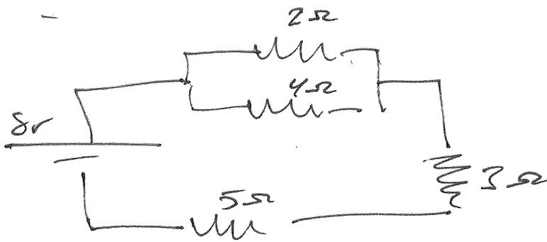
$$\textcircled{1} \quad \frac{1}{2} + \frac{1}{4} = \frac{1}{R_{\text{net}}} \quad \therefore R_{\text{net}} = 1.33 \Omega$$
